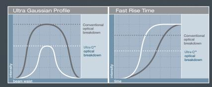
Ultra Q's Ultra Gaussian beam profile and fast rise time achieve optical breakdown (in air) of approximately 1.8mJ, in optimal conditions, compared to other YAG lasers, which typically achieve optical breakdown (in air) of 3 to 4mJ. This enables you to perform capsulotomy and iridotomy procedures at lower, more efficient power levels and with a reduced risk of side effects.
